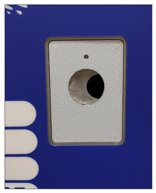
Using a hole saw or similar cut a 32mm hole though the inner door skin.
